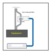
WARNING: If the SCT013 current probe jaws are not completely closed -- then the current measurement by the SYSTEM will be adversely affected. The SYSTEM will not operate and/or will operate inconsistently.
